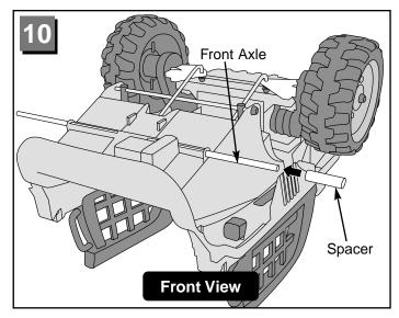
• Slide a spacer onto one end of the front axle.
